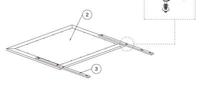
STEP 1: Fix Mirror Support on top of Mirror . Insert JCBC BOLT (A) into the holes at the mirror support . Tighten the support rail to the mirror & dresser with JCBC Bolt (A) using ALLEN KEY (D).
